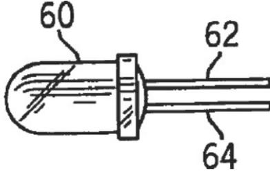
**DWPI Title:** Flashlight for e.g. civilian, has light emitting diode including two leads, and housing including side cover disposed on side of housing adjacent power source to enclose power source
